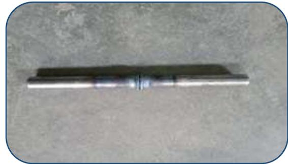
Gambar 5 Hasil *friction Welding* pipa baja
